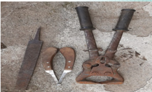
A picture showing from left to right the hoof file, hoof knives and hoof trimmer
