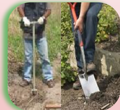
Sampling in the field using auger – left and tube – right.
